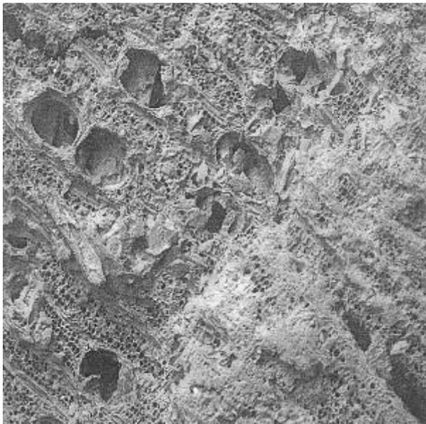
Figure 20. Cross section of waterlogged ash impregnated with 0.3 g/g PEG 2000 and freeze dried. The PEG is concentrated in the late wood and irregularly distributed in the early wood. Vessels are empty or filled with PEG. Maybe are tyloses are present in some of the vessels. Cracks are visible (50X)
