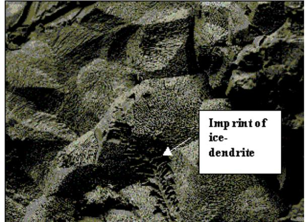
Figure 13. At the above image a largely eutectic mixture has been freeze-dried. This has left a maze of PEG lamellae in large hexagonal areas. An ice dendrite is seen in the lower part of the image indicating that there has been a small surplus of water relative to eutectic composition. (75X).
